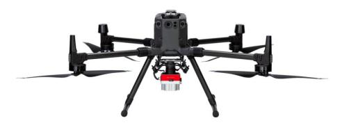
Altum-PT and DLS 2 on a Matrice 300. The sensor draws power directly from the Matrice via the Skyport.
